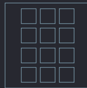
12x Modul 45° External dimension 243 x 243 mm
