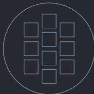
10x Modul 45° External dimension ∅ 294 mm
