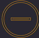
Tube body with handle clamp External dimension ∅ 140 mm
