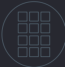
12x Modul 45° External dimension ∅ 324 mm
