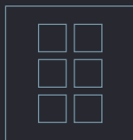
6x Modul 45° External dimension 222 x 222 mm
