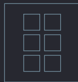
6x Modul 45° External dimension 199 x 199 mm
