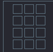
12x Modul 45° External dimension 243 x 243 mm
