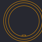
Blind plates External dimension ∅ 140 mm
