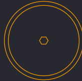
Blind plates External dimension ∅ 140 mm
