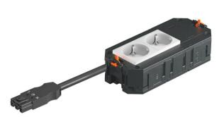
The ready-for-connection UTC3 universal support has 2 pre-installed 33° protective contact sockets in white of 16 A and one blanking cover for retroinstallation of an installation device of the Modul 45 or Modul 45connect series. Suitable for VL connection cables and device installation units of nominal size 2, 4, R4, 6 and R7.
