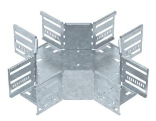
Cross-over for the creation of a horizontal branch, fitting for lock and screw-on cable trays of side height 85 mm. Screwless mounting with double clamps or screw connection with FRS truss-head screws and M6 combination nuts. Can be used indoors and outdoors. Fastening material must be ordered separately.
