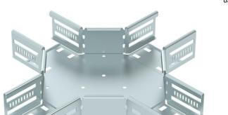
Cross-over for the creation of a horizontal branch, fitting for lock and screw-on cable trays of side height 60 mm. Screwless mounting with double clamps or screw connection with FRS truss-head screws and M6 combination nuts. Can be used in indoor areas. Fastening material must be ordered separately.
