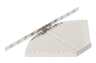
Angle-adjustable bend for the creation of a horizontal branch, fitting for lock and screw-on cable trays of side height 60 mm. Adjustable angle  $0-90^\circ$ . Screwless mounting with double clamps or screw connection with FRS truss-head screws and M6 combination nuts. Can be used indoors and outdoors. Fastening material must be ordered separately.
