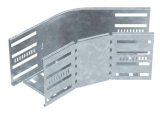
45° bend for the creation of a horizontal branch, fitting for lock and screw-on cable trays of side height 110 mm. Screwless mounting with double clamps or screw connection with FRS truss-head screws and M6 combination nuts. Can be used indoors and outdoors. Fastening material must be ordered separately.
