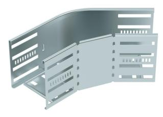
45° bend for the creation of a horizontal branch, fitting for lock and screw-on cable trays of side height 110 mm. Screwless mounting with double clamps or screw connection with FRS truss-head screws and M6 combination nuts. Can be used in indoor areas. Fastening material must be ordered separately.
