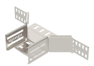
Add-on tee for the creation of a horizontal branch or cross-over, fitting for lock and screw-on cable trays of side height 60 mm. Screwless mounting with double clamps or screw connection with FRS truss-head screws and M6 combination nuts. Can be used indoors and outdoors. Fastening material must be ordered separately.
