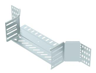
Add-on tee for the creation of a horizontal branch or cross-over, fitting for lock and screw-on cable trays of side height 110 mm. Screwless mounting with double clamps or screw connection with FRS truss-head screws and M6 combination nuts. Can be used in indoor areas. Fastening material must be ordered separately.
