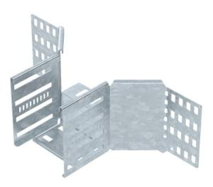
Add-on tee for the creation of a horizontal branch or cross-over, fitting for lock and screw-on cable trays of side height 110 mm. Screwless mounting with double clamps or screw connection with FRS truss-head screws and M6 combination nuts. Can be used indoors and outdoors. Fastening material must be ordered separately.
