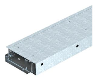
Ready-to-mount trunking unit for cable routing and device installation, consisting of a trunking base with two blanking covers and two adjustable floor covering contact profiles, for screed limitation in areas of door soffits and in front of radiator alcoves. The scope of delivery contains two lid butt seals and one connector.
