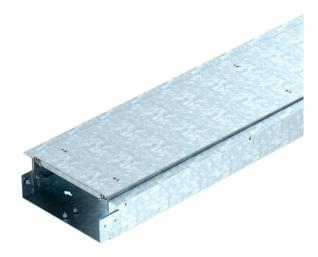
Ready-to-mount trunking unit for cable routing, consisting of a trunking base with two covers and two adjustable floor covering contact profiles, for screed limitation in areas of door soffits and in front of radiator alcoves. The scope of delivery contains two lid butt seals and one connector.
