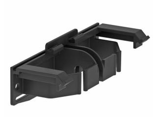
Cover adapter for mounting on trunking bases and fittings of the GAD and Rapid IBIS design device installation trunking series. The cover adapter can be pushed into a guide on the base and is used to accept the trunking cover and keep it at the desired spacing. It is also used for bundled cable exits and can be moved into the lengthwise direction. A maximum spacing of 500 mm between the cover adapters must be maintained.
